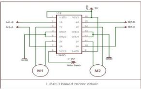
Figure: 3. Circuit diagram of dc motor driver
