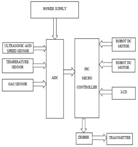
Figure: 1.Block diagram of transmitter
